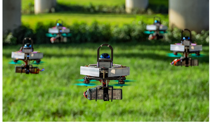
Fig. 1. An aerial swarm system constituted of five UAVs flying in the wild in which Swarm-LIO2 serves as the self and mutual state estimator. More details can be found in the attached video at https://youtu.be/Q7cJ9iRhly
