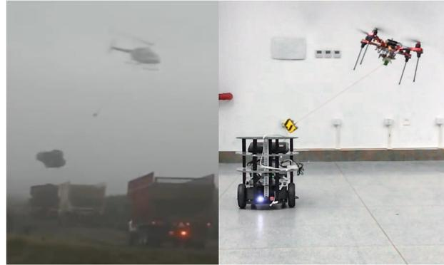
Fig. 1. Experienced helicopter pilot transporting Christmas tree (left). Autonomous MAV throwing payload precisely to a moving vehicle, using our estimation system (right).
